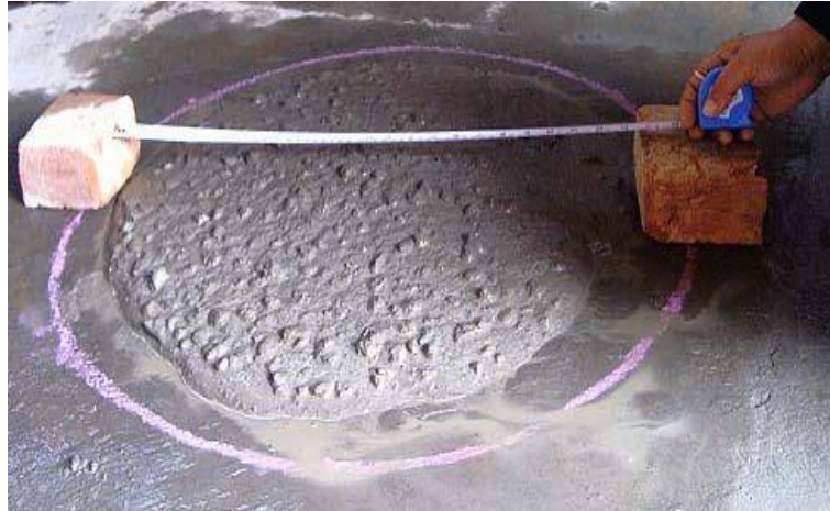
Figure 1. Slump Flow Test
